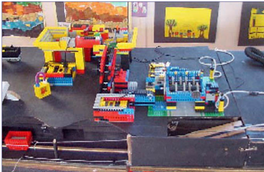
Figure 8: Crusher on the right with a conveyor belt taking the coal over to the main conveyor belt where it is being taken up to the sorting towers. The programmable bricks have been enclosed in a different coloured casing for easy identification by the different groups.
